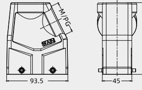
Suitable for cable with maximum OD Ø32mm
